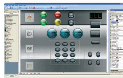
Stardraw Control Forms View showing CD UI Form
